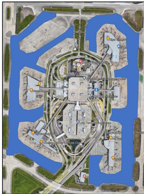
Blue areas depict the apron in which pedestrians are not allowed to transverse unless actively involved in an aircraft pushback or engaged in an activity
