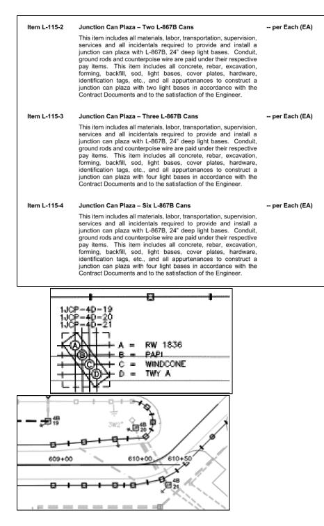
R.2 Only 2-can and 4-can junction can plazas are required for this Project. Refer to attached revised Drawings E301 through E307, A Airfield Lighting Circuiting Plans (attached to this Addendum No. 2) for additional clarification and enlarged junction can plaza information.
