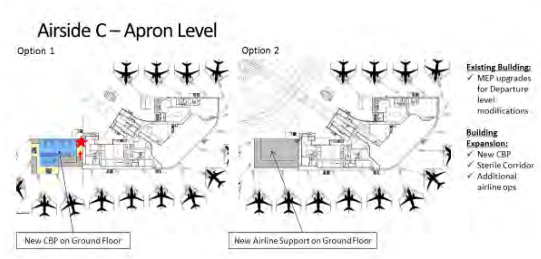
Figure 5.74 Airside C Expansion Options – Apron Level
