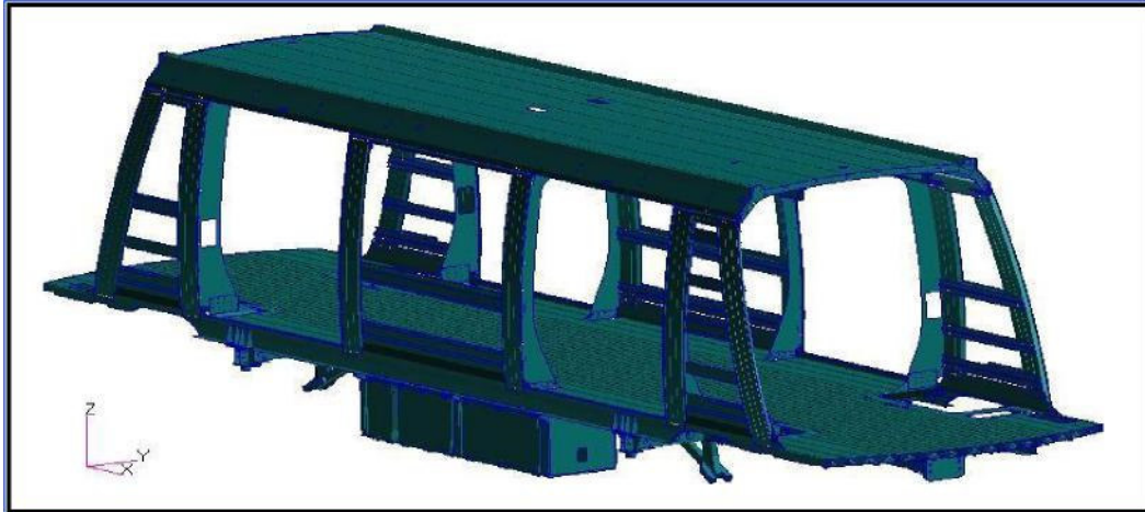
Figure 2: Car body FEA model example
