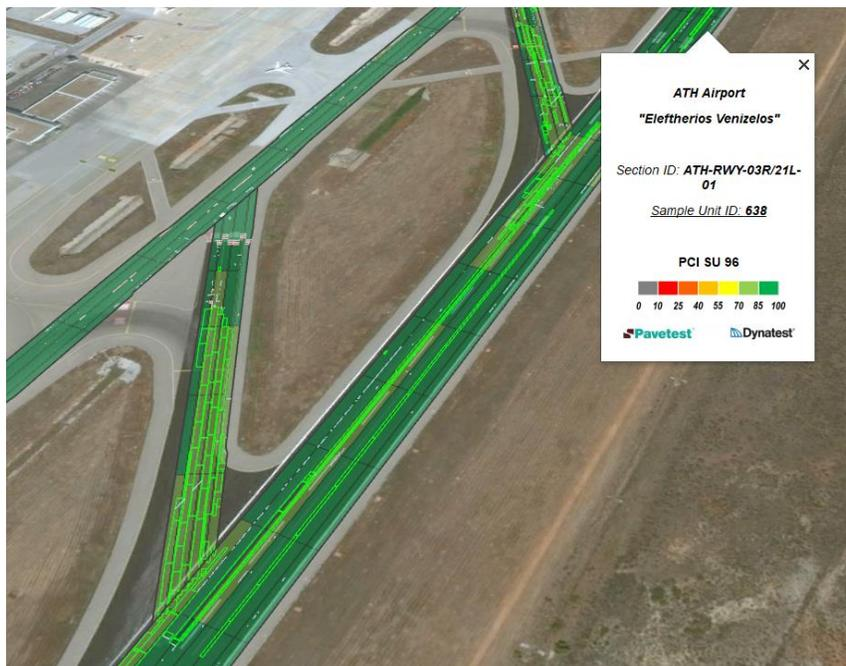
Figure 8 PCI Data and Distresses on Asphalt Pavements
