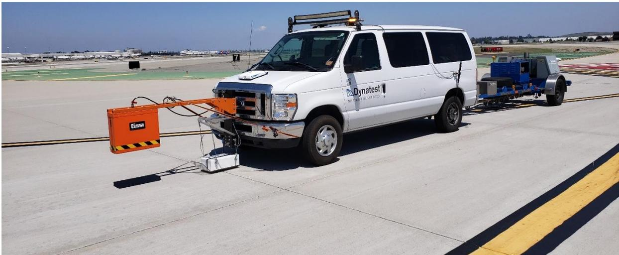
Figure 14 ARA HWD integrated with a GPR
