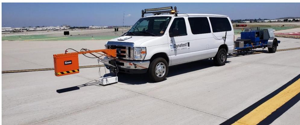
**Figure 1. ARA HWD integrated with a GPR**
