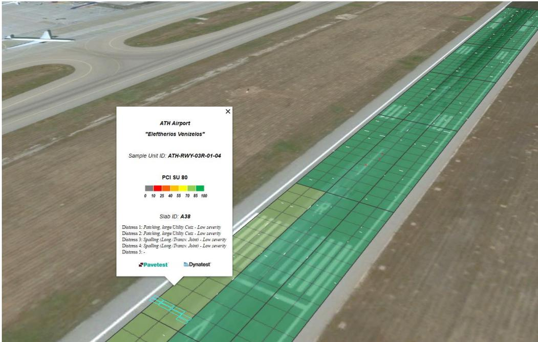
Figure 7 PCI Data and Distresses on Concrete Pavements
