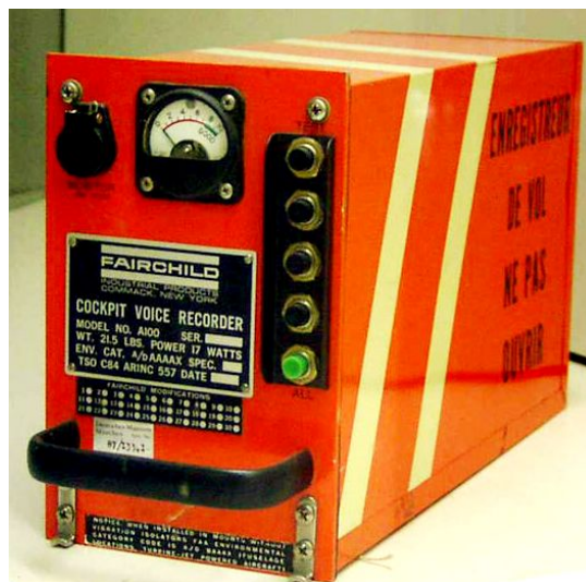
Figure 2. Representative Cockpit Voice Recorder
