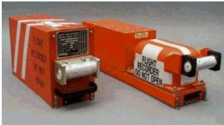
Figure 1. Representative Flight Data Recorders
